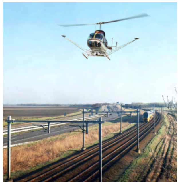
Specially modified aircraft are fitted with sensors that include photographic and LiDAR distance measurement equipment.
